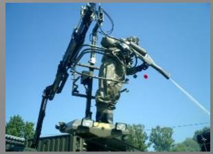
Pallet crane with basket for vehicle decontamination
